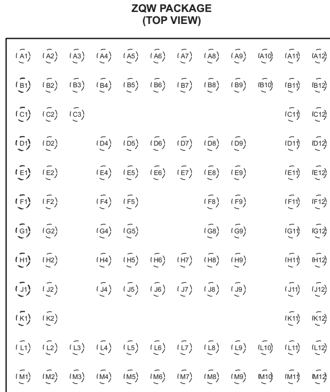
Figure 4-3. 113-Pin ZQW Package (Top View), MSP430FG6626IZQW, MSP430FG6625IZQW, MSP430FG6426IZQW, MSP430FG6425IZQW
